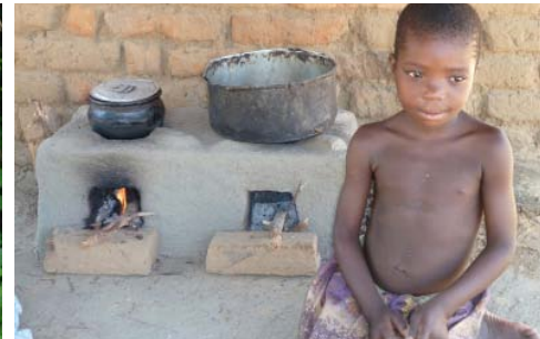
The fire is contained and is at the side of the kitchen, making it safer and providing more space. The Changu Changu Moto also produces less smoke
