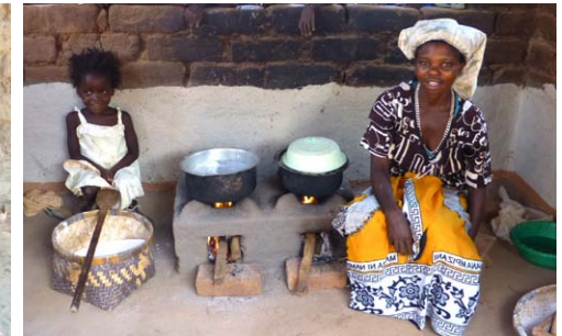
The Changu Changu Moto only uses small amounts of wood, is much more efficient and cleaner to use, and benefits from a double burner
